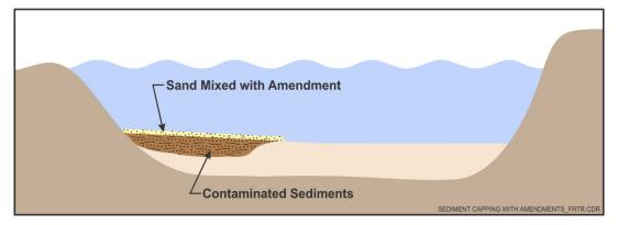
Cross Section of Sediment Capping with Amendments
